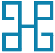
BOTTOM TRACK TWO TRACK WITH MOSQUITO 338-0426 1.33 Kg/M
